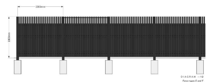
The fencing along Pardoa Boulevard is designed to be visually appealing from the street while still providing noise attenuation within the back yards of adjoining properties. The fence is to be built lot by lot and allowance for the fence to continue at either end is required. No Plywood backing is required when the fence is side on to Pardoa Boulevard against an open space link.
