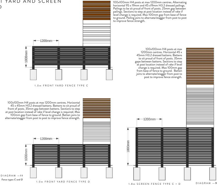
Note: All gate posts on 1.8m type C or D screen fence returns to be 112.5 x 112.5mm H5 glue laminate timber to prevent twisting.
