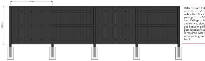
100x100mm H4 posts at max 2000mm centres. 100x50mm H3.2 rough sawn rails with 150 x 25mm H3.2 rough sawn pailings. 100 x 50mm H3.2 rough sawn cap. Pailings to be flush with front of posts and to swap sides at each post. 5-10mm gap between pailings. Sections to step at post location instead of rake if level change is required. Max 100mm gap from base of fence to ground. Fence to be painted black.
