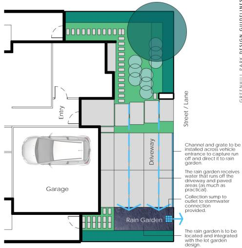
$\begin{array}{l} {\sf DIAGRAM} \ - {\sf 21} \\ {\sf Rain \ Garden \ Typical \ Location} \end{array}$
